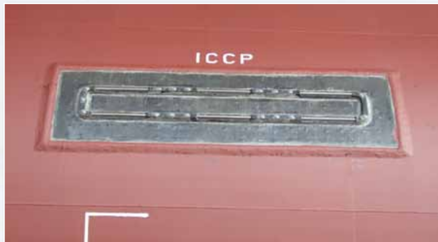
Linear loop anode with di-electric shield
