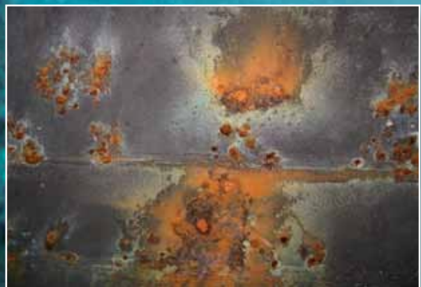
Corrosion 'blisters' on hull plate.
