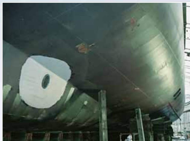
Elliptical anode with di-electric shield
